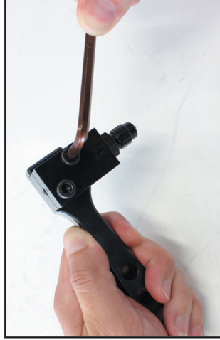
STEP 2: Using the 5mm allen key supplied, unscrew the 2 x 5mm SHCS half a turn.
