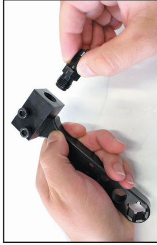
STEP 1: Screw in the STOP adapter completely until hex bottoms out against tool.
