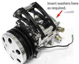
4. Fit bracket assembly to Sanden compressor and slide long bolt through compressor ears and secure with nut supplied. insert washers between bracket and compressor ear.
