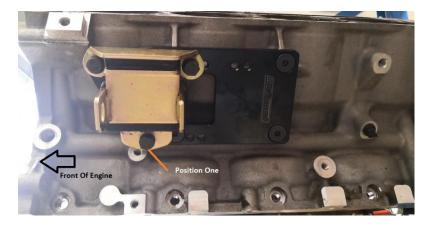
Position One: Places the LS engine in the stock SBC location
