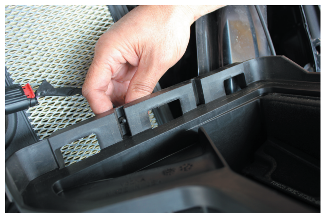
11. The mass air flow sensor is held in with a christmas tree clip. Use long nose pliers to gently squeeze it back through the hole.
