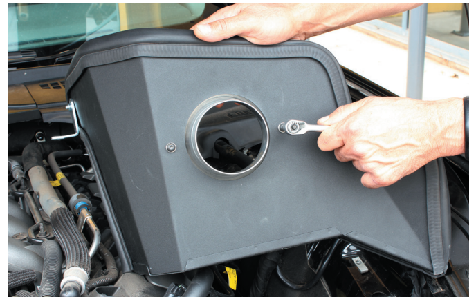
17. Secure filter adapter with the included hardware.
