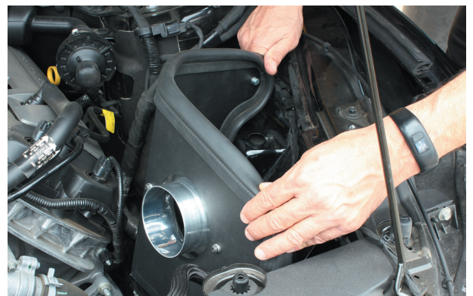
19. Slip the heat shield into place and line up the mounting holes to the brackets
