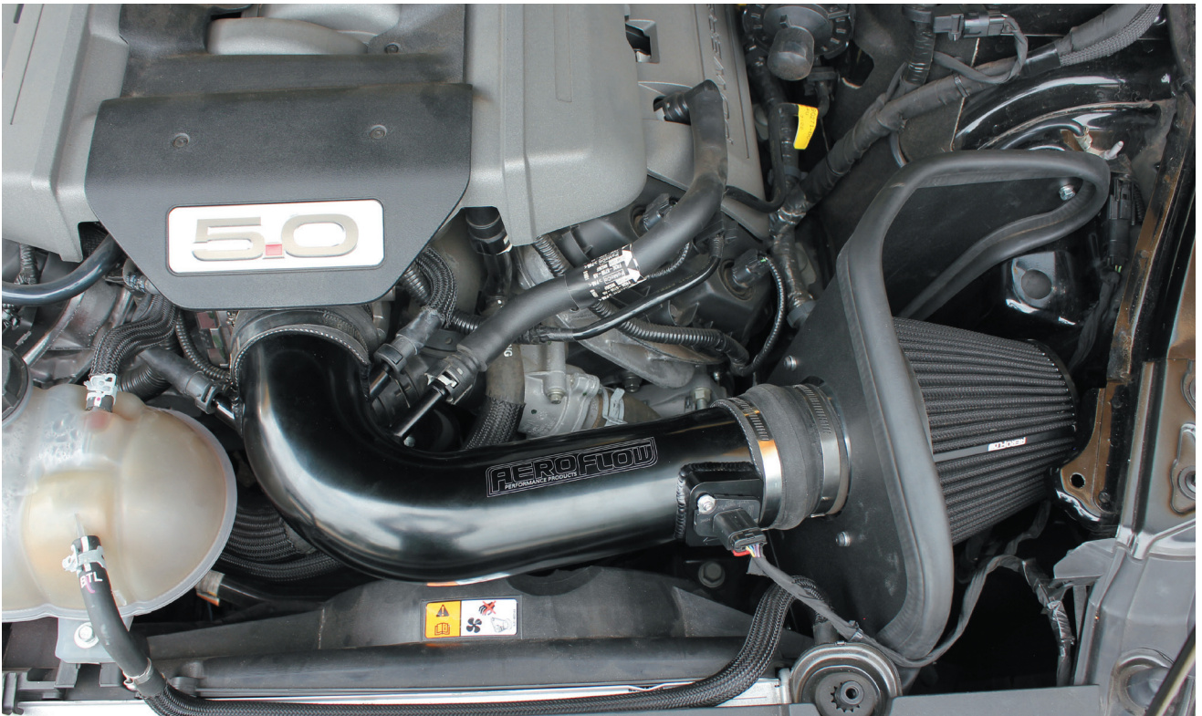
29. Reconnect all factory hoses to the intake tube and double check all fittings and bolts are tight. We hope you enjoy your AeroFlow cold air induction kit.
