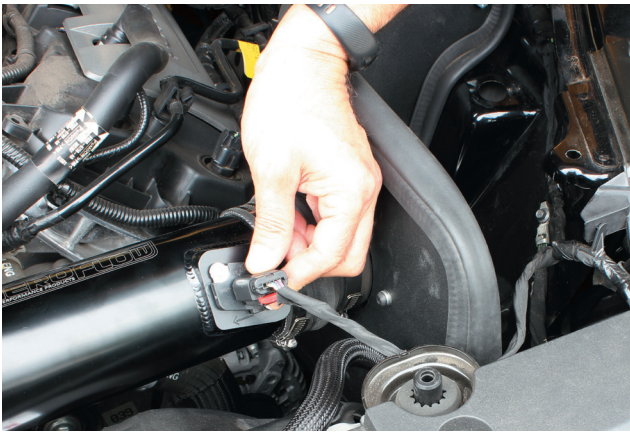
27. Reconnect the mass air flow sensor.
