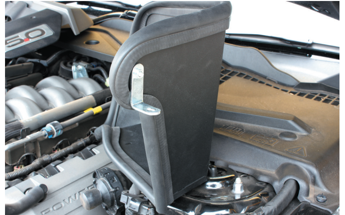
15. Install the small L bracket to the top left hand hole on the shield. Be sure to use the spacer between the bracket & shield.
