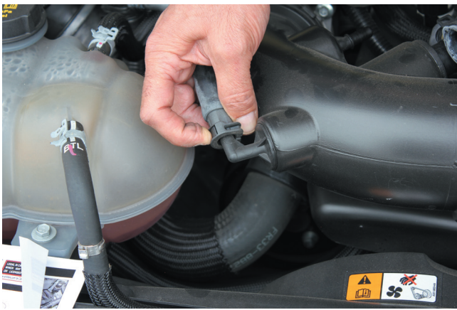
4. Unclip the left hand idle bypass hose by pressing on the clip
