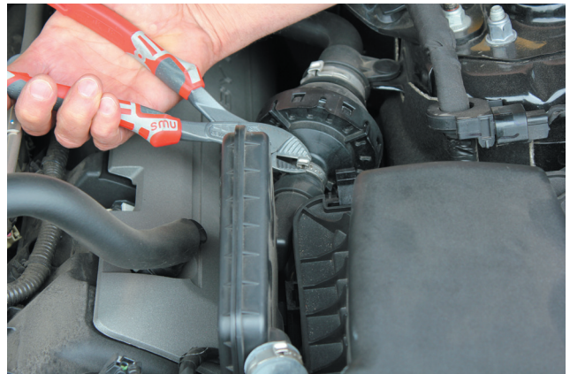
7. Cut off the clip on the sound drum and remove the hose and chamber in front of the drum.
