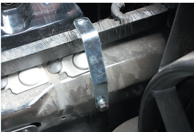
18. Install the longer L bracket to the chassis rail with the larger bolt washer and spring washer supplied
