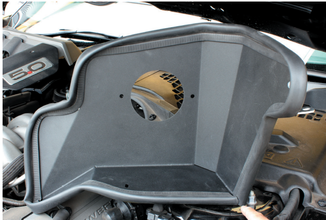
14. Take the steel heat deflector in your kit and install the included rubber, starting in the indicated corner, cut to fit.
