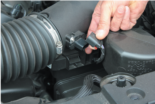
6. Unplug the mass air sensor by sliding back the red locking tab and sliding the plug off.
