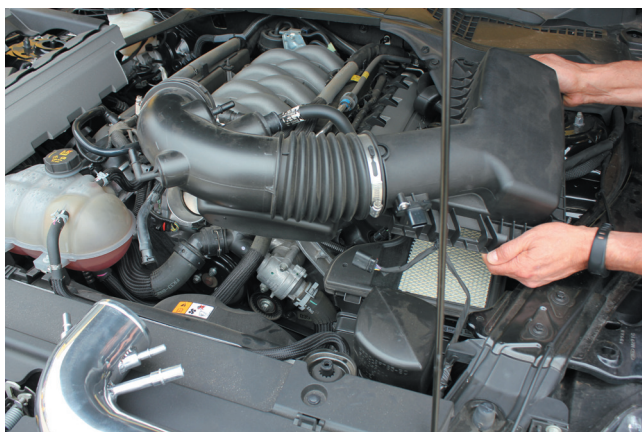
10. At this point you can unclip the air box and remove the entire top section.
