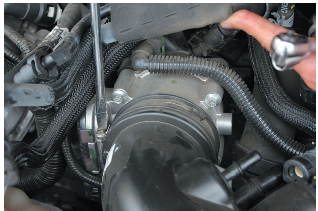
9. Loosen the clamp on the throttle body holding the intake tube on.
