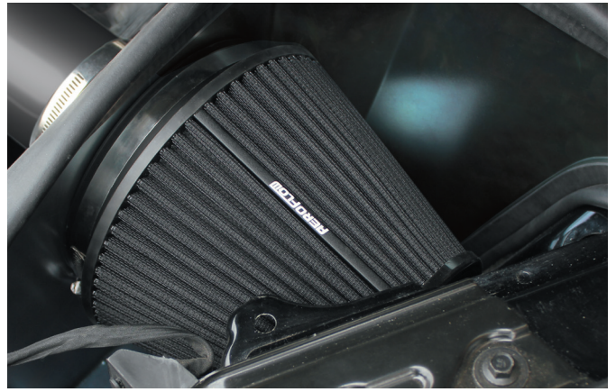
28. Gently manoeuvre the AeroFlow air filter onto the air filter adapter and secure with the supplied hose clamp.
