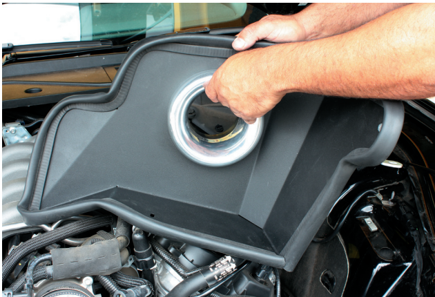
16. Fit the filter adapter to the shield
