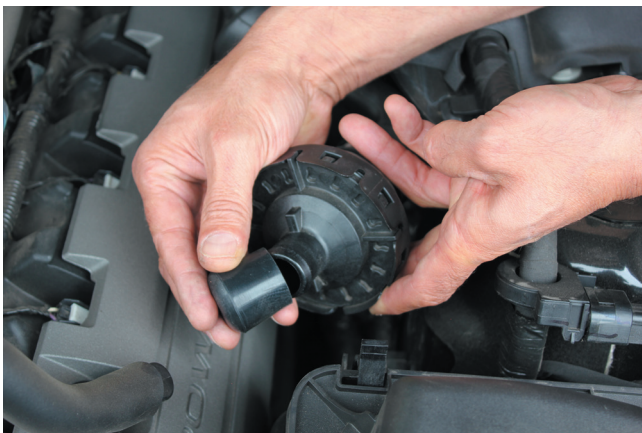
8. Install the supplied rubber cover on the front of the sound drum.
