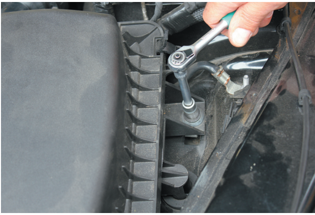
12. Unclip the lid of the original air box and remove. Unbolt the original air box bottom section.
