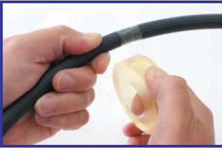
1. Measure desired hose length and wrap tightly with Aeroflow's non-stick cutting film, (part # AF98-2049), allowing at least 3 full rotations of the non-stick film.
