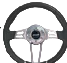
GR457 Club Sport Model. The wheel rims are molded self skin polyurethane with a textured leather grain finish and polished accents. The spokes are polished aluminium with a clear anodized finish. The wheels have polished trim rings. 13 1/2" diameter, 3 1/2" dish including styling sleeve.
