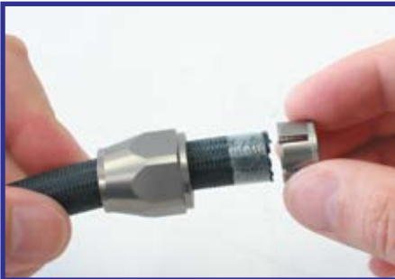
4. Carefully slide the olive onto the end of the hose ensuring that the slots in the olive face towards the socket nut.
