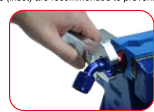
Tighten the fitting until the socket has a gap of approximately 1.5mm. Check that the mark on the hose has not moved from the end of the socket nut.
