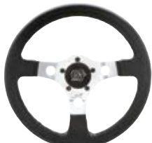
GR457 Club Sport Model. The wheel rims are molded self skin polyurethane with a textured leather grain finish and polished accents. The spokes are polished aluminium with a clear anodized finish. The wheels have polished trim rings. 13 1/2" diameter, 3 1/2" dish including styling sleeve.
