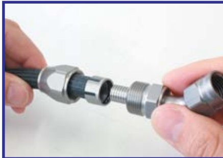
5. Carefully slide olive past non-stick film then remove the non-stick film and slide olive back up to end of hose. Apply a small amount of Aero-Seal (part # AF98-2023), onto the male thread of the kryptalon® hose end and screw the socket nut onto the Kryptalon® hose end.
