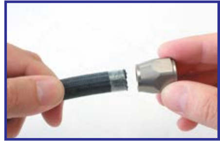
3. Carefully slide the socket nut over the hose while keeping the non-stick film on the end of the hose.
