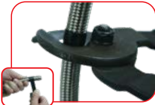
Wrap masking or electrical tape tightly around the hose to prevent fraying and cut with hose cutters for best results.
