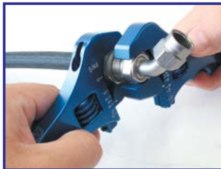
6. Secure the hose end socket using Aeroflow vice jaws (part # AF98-2001 or AF98-2002) or by using an Aeroflow aluminium wrench (part # AF98-2003 or AF98-2039). Tighten the Kryptalon® hose end clockwise until the socket nut is tight, ensuring the correct crush of the olive onto the hose. You should notice that the male thread of the fitting is not showing, covered by the socket nut.
