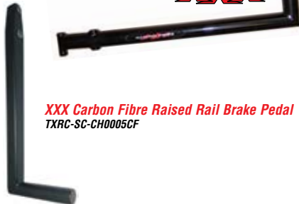
XXX Brake Pedal Raised Rail Black powdercoated 4130 Chromoly pedal to suit raised rail cars. 13" Long from chassis pivot to bottom. 2-3/8" centre - centre from chassis pivot to master cylinder spud. 5" wide. Weight: 0.4 lbs TXRC-SC-CH-0005
