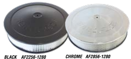
BLACK AF2256-1280 CHROME AF2856-1280 14" X 3" (355.6mm X 76.2mm) 1-1/8" (28mm) Drop base 5-1/8" (130mm) neck with paper element. Replacement element AF2046-2110 95mm (3-47/64") total height.
