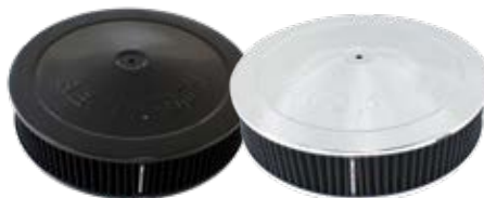
AF2251-1280 Black Air Cleaner Assembly 14" X 3" (355.6mm X 76.2mm), 1-1/8" (28mm) Drop base 5-1/8" (130mm) neck with black reusable/washable element. Replacement element AF2041-1650 95mm (3-47/64") total height. AF2851-1280 Chrome Air Cleaner Assembly
