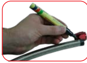
Mark the hose with a felt pen to detect any movement while the assembly process is completed.
