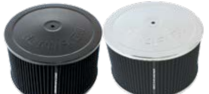
AF2251-1365 Black Air Cleaner Assembly 9" x 5" (228.6mm x 127mm) 5-1/8" (130mm) neck with black reusable/washable element Replacement element AF2041-3650 153mm (6") total height. AF2851-1365 Chrome Air Cleaner Assembly
