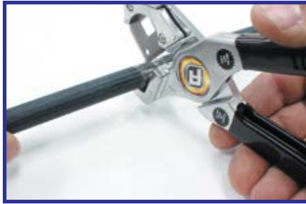
2. Cut through the center of non-stick film while ensuring that you cut the hose at a 90 degree angle using Aeroflow cutters, (part # AF98-2052), or alternatively you can use a box cutting knife being careful not to fray the Kevlar braid.
