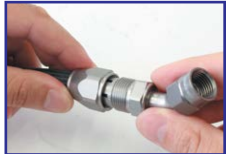
5. Carefully slide olive past non-stick film then remove the non-stick film and slide olive back up to end of hose. Apply a small amount of Aero-Seal (part # AF98-2023), onto the male thread of the kryptalon® hose end and screw the socket nut onto the Kryptalon® hose end.
