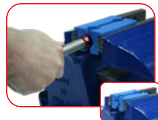
Place the socket in a vice, remove the tape from the hose and push it into the nut while twisting the hose. Aeroflow's soft jaw vice adapters (inset) are recommended to prevent damage to fittings.
