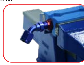
Holding the hose, push the socket nut onto the nipple thread.
