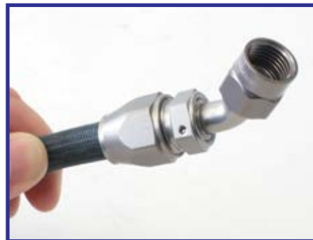
6. Secure the hose end socket using Aeroflow vice jaws (part # AF98-2001 or AF98-2002) or by using an Aeroflow aluminium wrench (part # AF98-2003 or AF98-2039). Tighten the Kryptalon® hose end clockwise until the socket nut is tight, ensuring the correct crush of the olive onto the hose. You should notice that the male thread of the fitting is not showing, covered by the socket nut.
